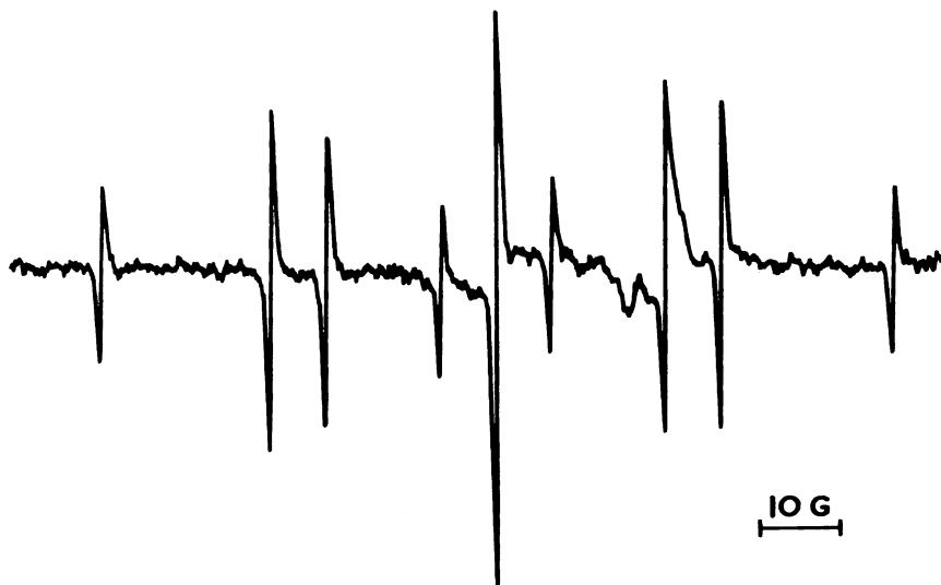
Figure 2. ESR spectrum of the propyl radical obtained by the photolysis of di- tert -butyl peroxide in the presence of tripropyltin chloride: t\text{-BuO}\cdot + \text{Pr}_3\text{SnCl} \rightarrow t\text{-BuOSnPr}_2\text{Cl} + \text{CH}_3\text{CH}_2\text{CH}_2\cdot
