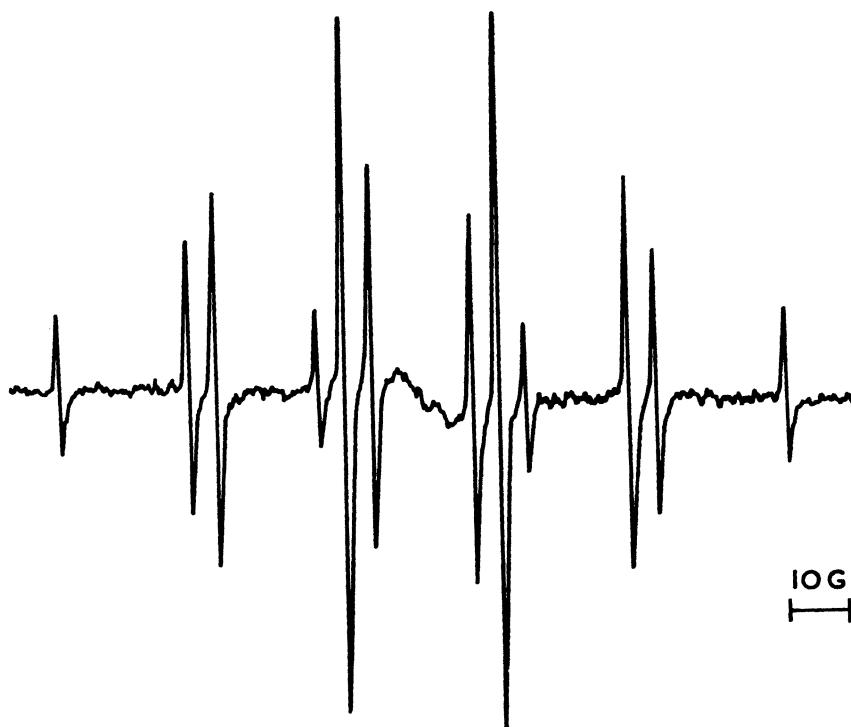
Figure 1. ESR spectrum of the ethyl radical obtained from the photolysis of di-tert-butyl peroxide and hexamethylditin in the presence of ethyl bromide (3): \text{CH}_3\text{CH}_2\text{Br} + \text{Me}_3\text{Sn}\cdot \rightarrow \text{Me}_3\text{SnBr} + \text{CH}_3\text{CH}_2\cdot
